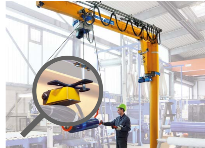
Limit switch for cross travel (Fig. 8)
