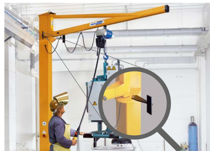
Slewing limit stops, adjustable (Fig. 5)
