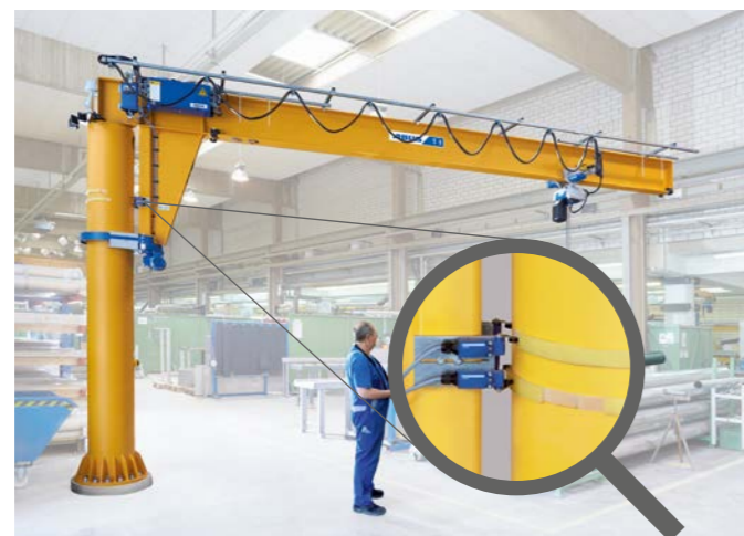
Slewing limit switch, VS (Fig. 6)
