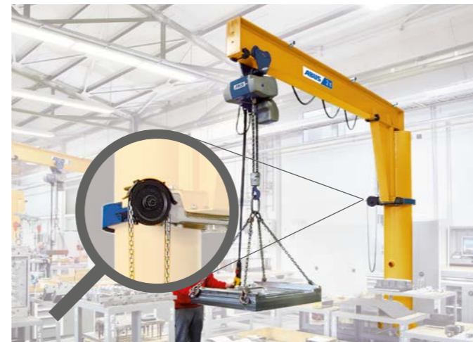
Adjustable brake, VS (Fig. 9)
