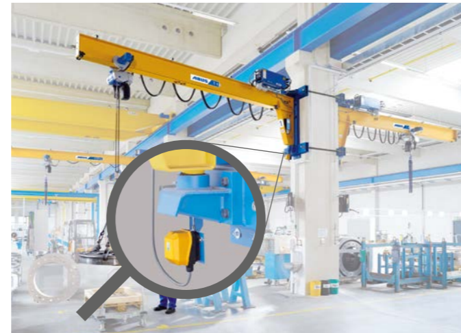
Slewing limit switch, VW (Fig. 7)
