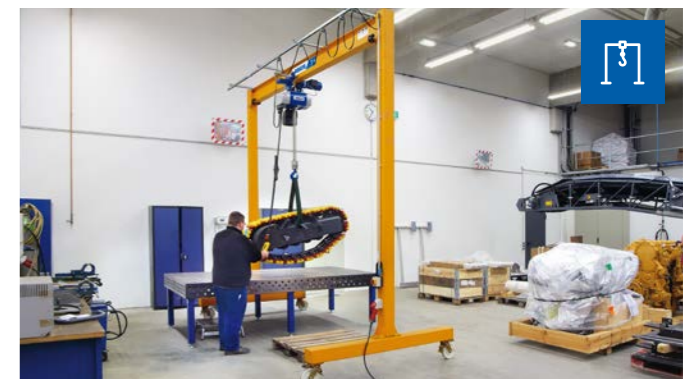
Lightweight mobile gantry LPK
